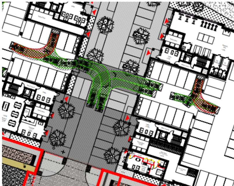
Extract from submitted tracking drawing showing ingress/egress from podium parking access points entrances from of central access road
