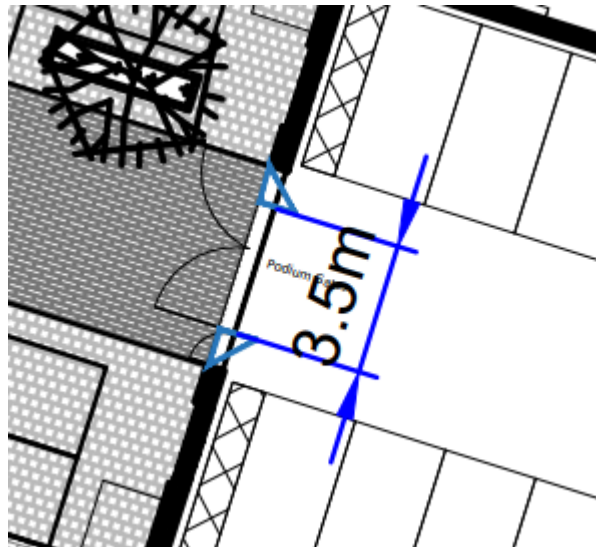
Extract from pedestrian visibility splay drawing showing 1m x 1m vision splays at podium access point off central access road.
