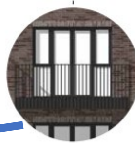
Projecting balconies with laser cut decorative balustrade
