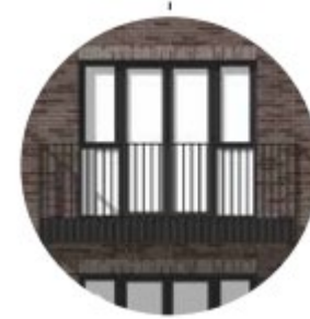
Projecting balconies with laser cut decorative balustrade
